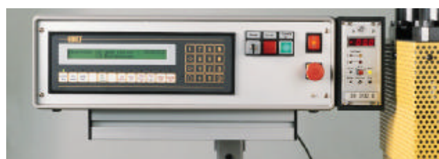
Electronic control of press-in force and board thickness
