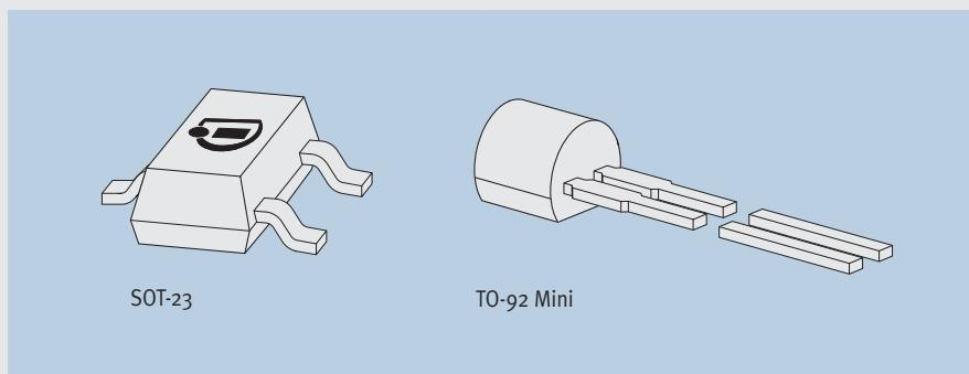
Temperature sensing has in the past predominantly been the domain of PTC Thermistors. Infineon Technologies offers with the KT-Series Silicon Temperature Sensor a cost competitive alternative.
